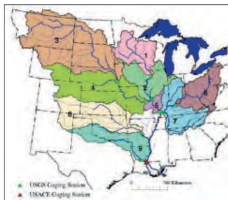
**Location** of nine large sub-basins comprising the MARB that are used for estimating nutrient fluxes (from Aulenbach et al., 2007).
